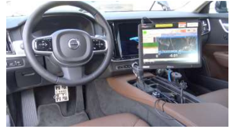
Vehicle that can be controlled by ABD electronics without physical actuators
