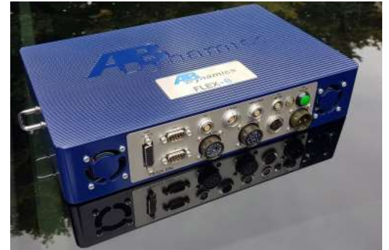
Flex-0 – Direct control of vehicle actuators
